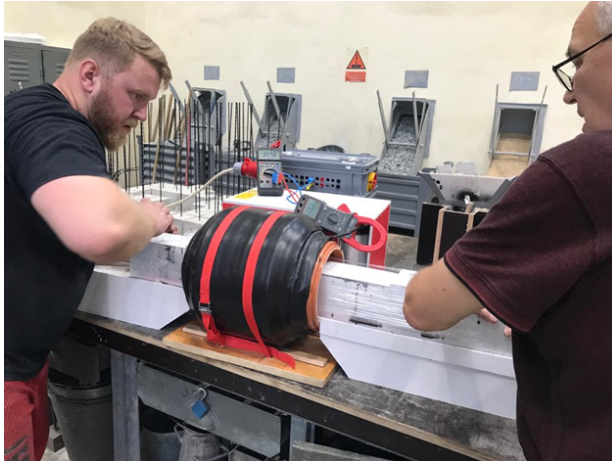
FIGURE 3. Pulling a filled mould through the device.
