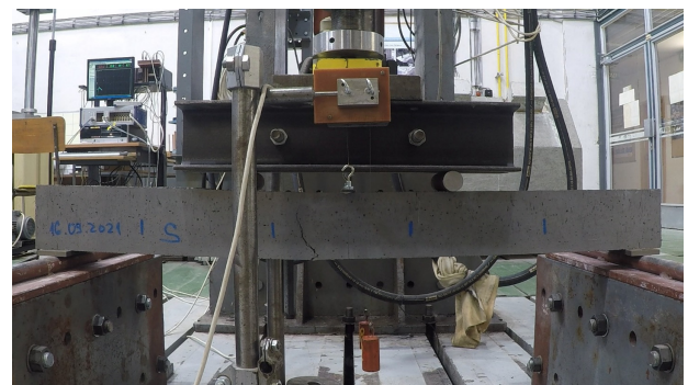
FIGURE 5. Four-point bending test setup.
