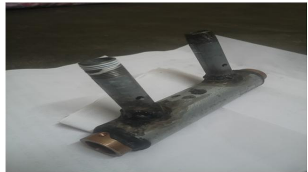
FIGURE 10. Assembly of the inner and outer pipe.
