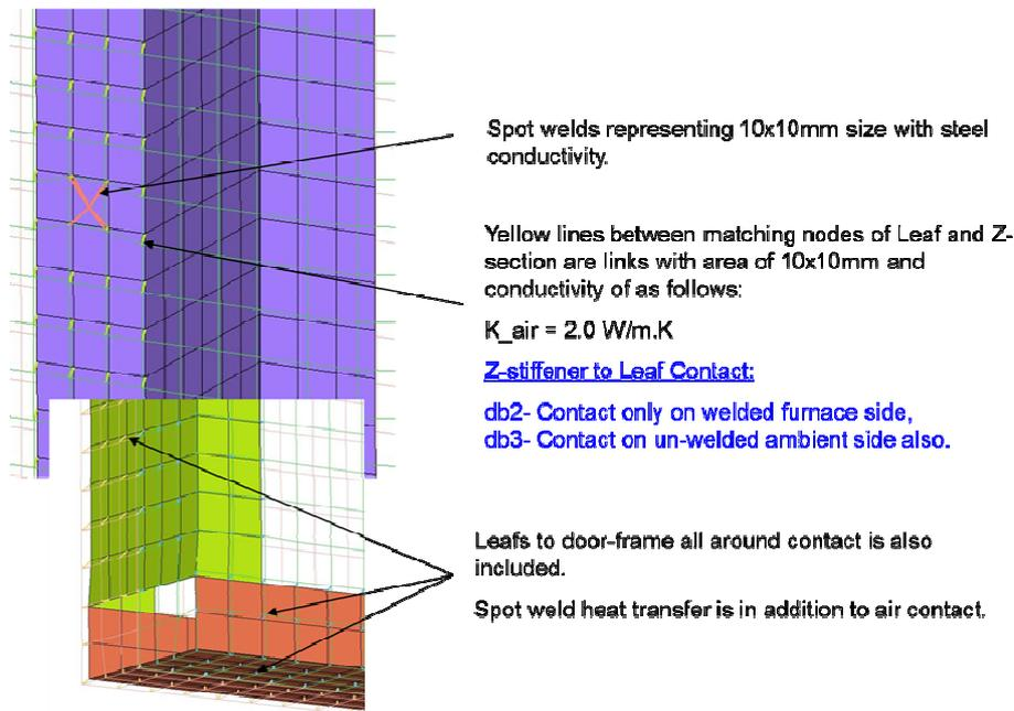
Fig. 5 Description of different thermal contact configurations
