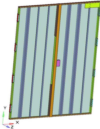
Fig. 3 Solid model of double steel fire door
