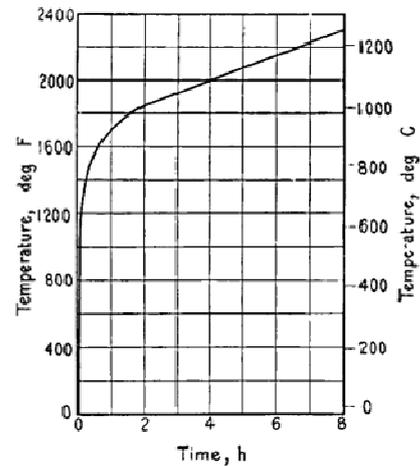
Fig.2 Standard time-temperature curve
