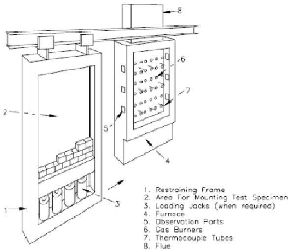
Fig. 1 Schematic of Setup
