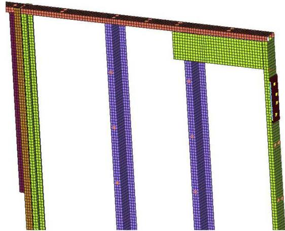
Fig. 4 Detail of connection in FE model
