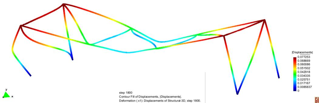
Fig. 9. Structure deformation @ 1800s, 20 mm slit for columns
