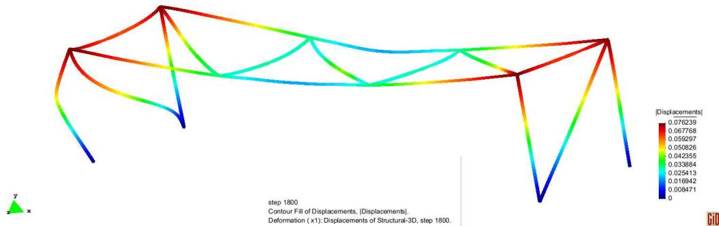
Fig. 10. Structure deformation @ 1800s, 200 mm slit for columns
