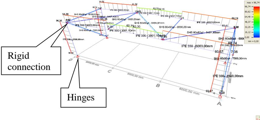
Fig. 2. Reference case, unity check at ambient temperature
