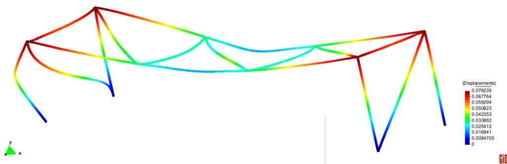
Fig. 11. Structure deformation @ 1800s, 20 mm slit for columns
