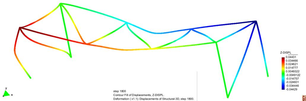
Fig. 8. Structure deformation @ 1800s, 200 mm slit for columns
