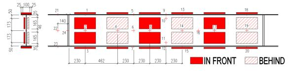
Fig. 8 Layout of flexible ceramic pads and thermocouples
