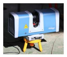
Fig. 6 Laser scanner
