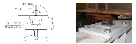
Fig. 4 Fixed pin point support
