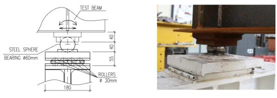
Fig. 5 Free pin point support
