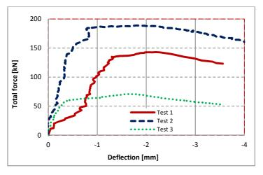
Fig. 13 Horizontal deflection of bottom flange at midspan
