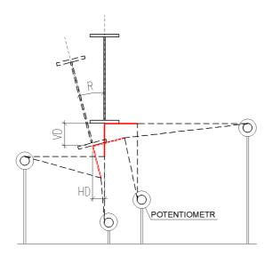
Fig. 9 Measuring of displacement at midspan
