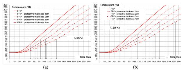
Fig. 9: Temperature in FRP on the top side (a) normal (b) heat-resistant resins
