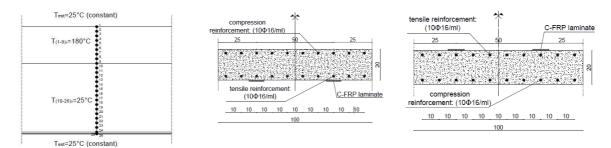
Fig. 3Slab discretization
