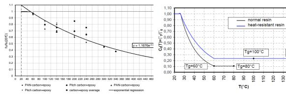
Fig. 1Temperature-dependent tensile strength reduction of various carbon fibre composites.
