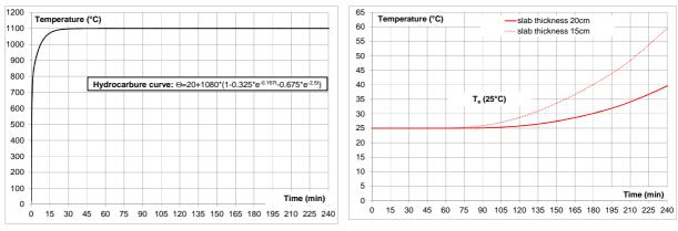
Fig. 7 Nominal Temperature-Time fire curves
