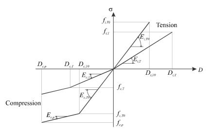
Fig. 3 Stress-strain relationship for timber at ambient and elevated temperature
