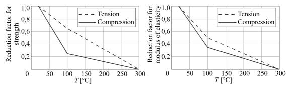
Fig. 2 Reduction factor for strength and modulus of elasticity parallel to the grain of softwood (EN 1995-1-2 (2005))
