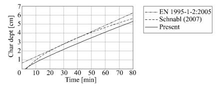
Fig. 4 Comparison of different one-dimensional charring models
