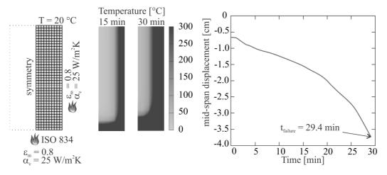
Fig. 6 Finite element mesh, temperature distribution in the cross-section and the timedisplacement curve of the analyzed timber beam
