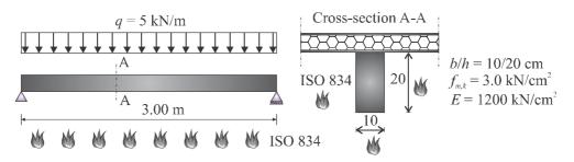
Fig. 5 Data for simply-supported timber beam
