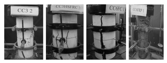
Fig. 3 Failure pattern of heat damaged cylinder and strengthened specimens
