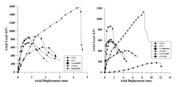
Fig. 6 Comparison of control and heat damaged specimens with 600°C strengthened cylinders
