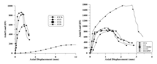
Fig. 4 Axial load- displacement comparison of control and heat damaged cylinders
