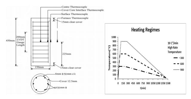
Fig. 1 Reinforcement details and position of thermocouple
