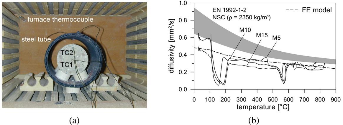
Fig. 1 (a) Cylinders inside the electric furnace instrumented with 2 thermocouples (TC1 and TC2); and (b) thermal diffusivity versus temperature
