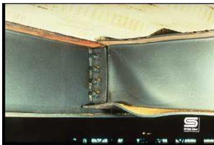
Fig. 1 Shear buckling and bottom-flange buckling in Cardington fire test (Newman et al., 2000)
