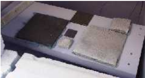
Fig. 2. Plates after fire test
