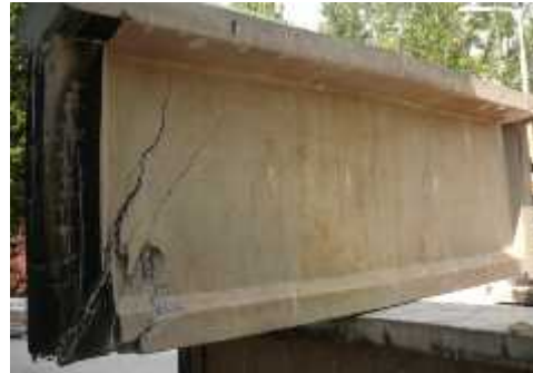
Fig.5 Beam No. 3 (Mix 4) after the web failure in shear
