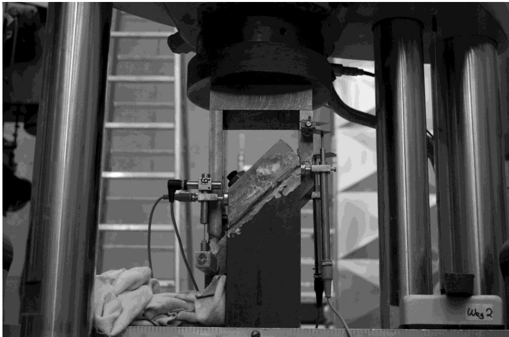
Fig. 5 Prototype of the new test rig for an angle of 45°
