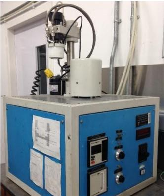
Fig. 6 Heat flow meter
