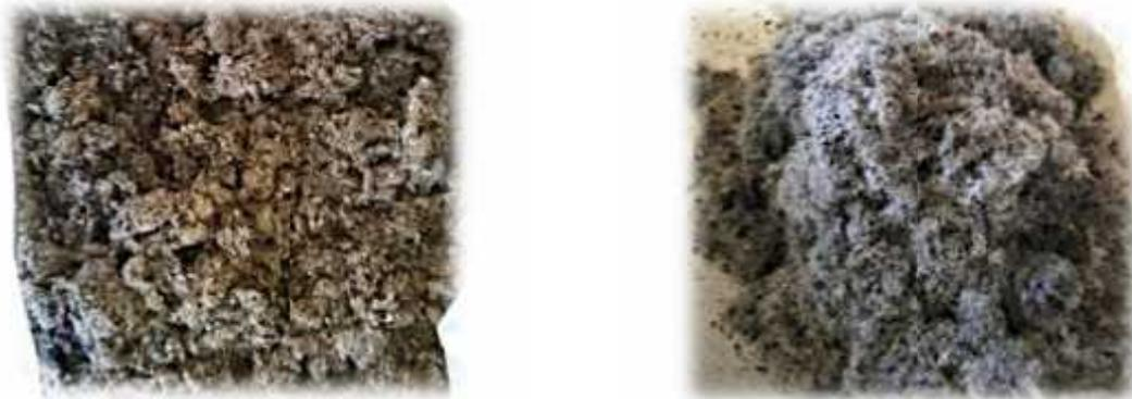
Fig. 2 Tyre polymer fibres before (left) and after (right) processing for reuse
