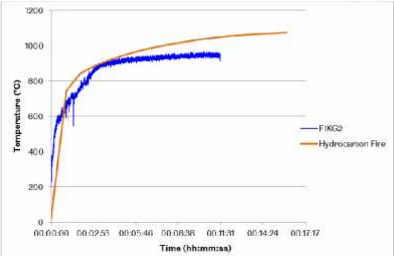
Fig. 6 Surface temperature of F1KG2 vs. hydrocarbon fire
