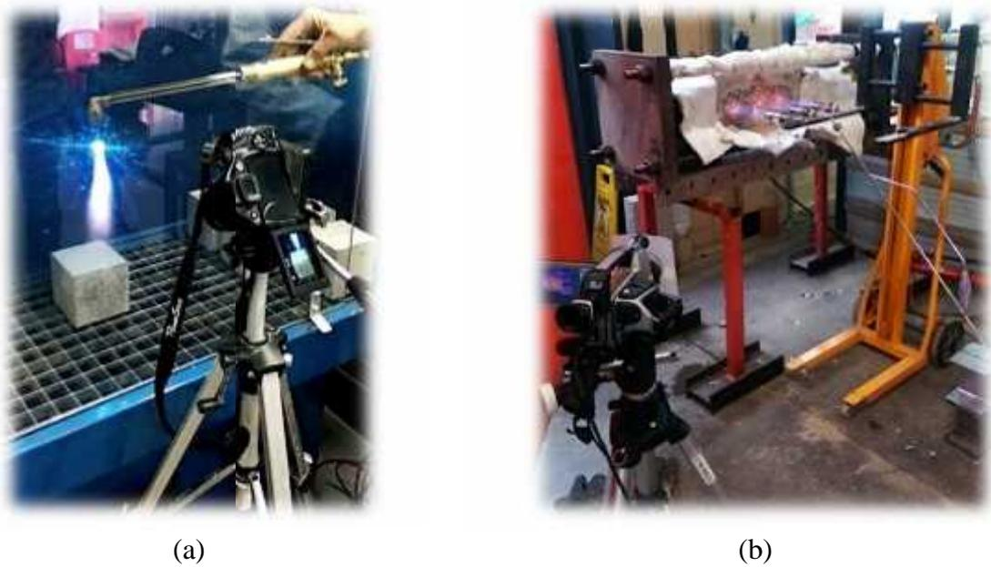
Fig. 3 Test setup (a) cube tests, (b) slab tests
