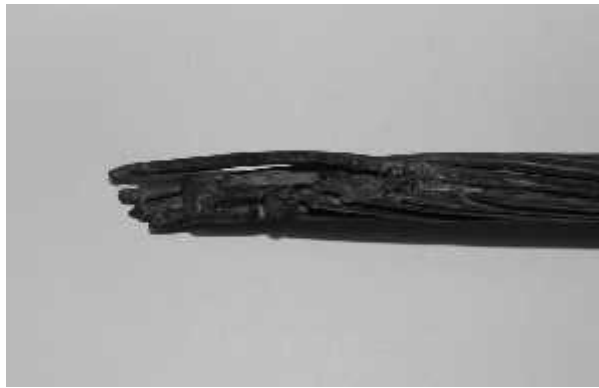
Fig. 7 Traces of the secondary short circuit at the end of the wire
