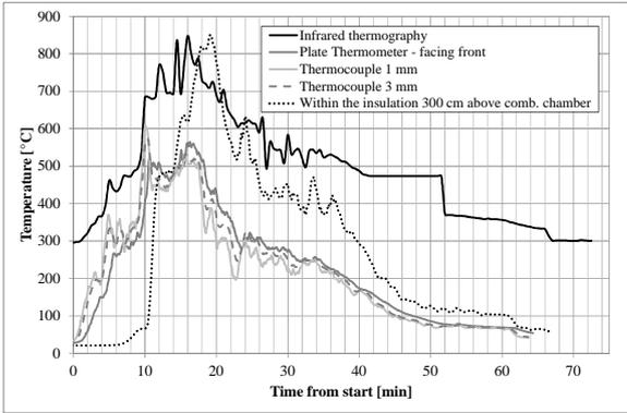
Fig. 4 Temperature at 250 cm above combustion chamber - EPS
