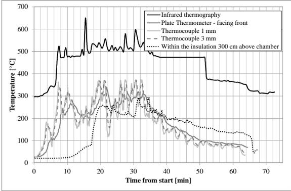
Fig. 6 Temperature at 250 cm above combustion chamber - EPS+MW
