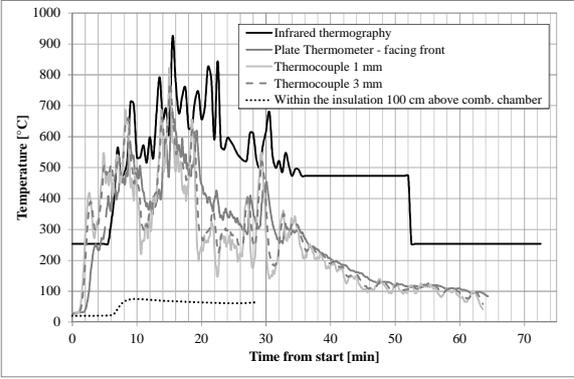
Fig. 7 Temperature at 125 cm above combustion chamber - MW
