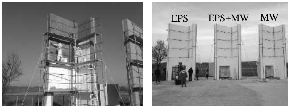
Fig. 1 Erecting the specimens (left), finished specimens (right)
