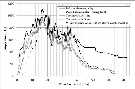
Fig. 3 Temperature at 125 cm above combustion chamber - EPS
