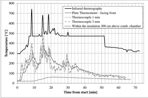
Fig. 8 Temperature at 250 cm above combustion chamber - MW
