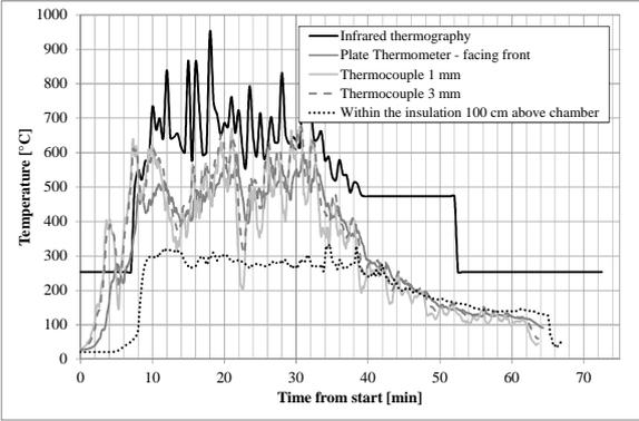
Fig. 5 Temperature at 125 cm above combustion chamber - EPS+MW
