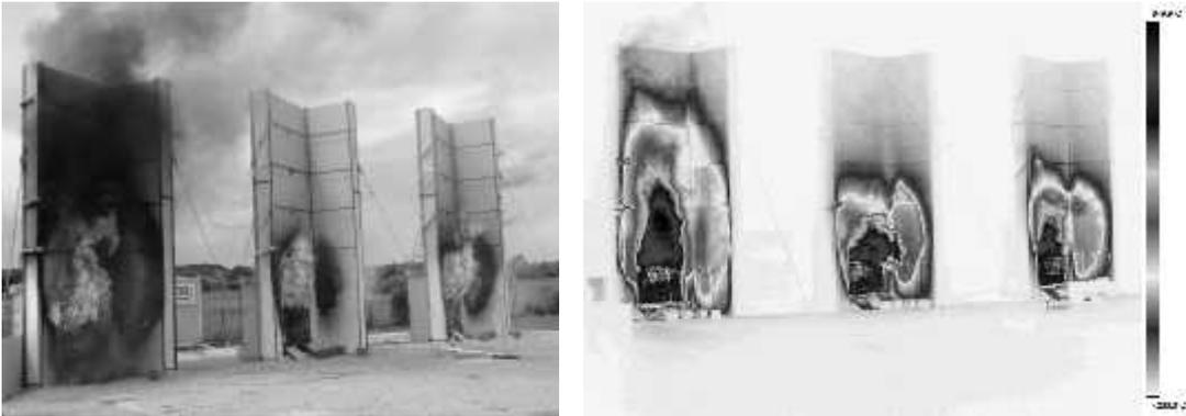
Fig. 2 Photography (left) and thermogram (right) of the tested specimens
