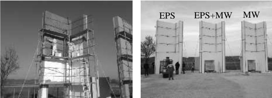
Fig. 1 Erecting the specimens (left), finished specimens (right)
