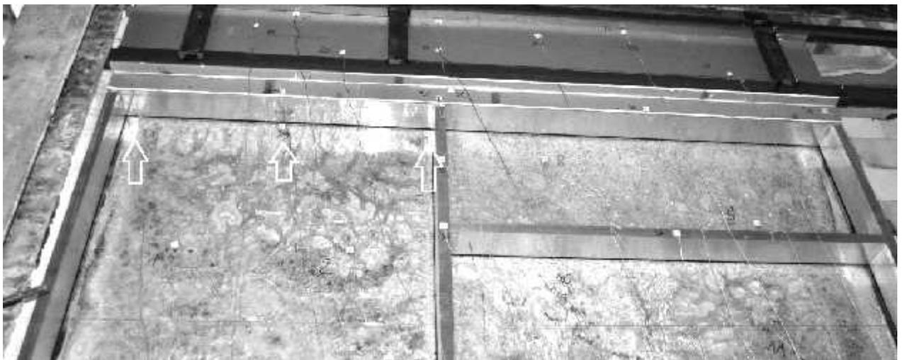
Fig. 6 Additional thermocouples placement in fire resistance test of curtain wall, test 3
