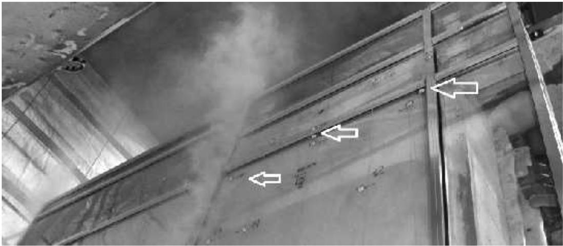
Fig. 4 Additional thermocouples placement in fire resistance test of curtain wall, test 2
