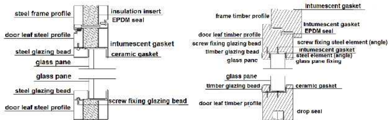
Fig. 1 An exemplary cross-sections of the steel and timber profile (Izydorczyk et al., 2014)
