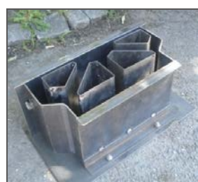
Figure 5 Moulds for concrete blocks Figure 6 Dimensions of blocks
