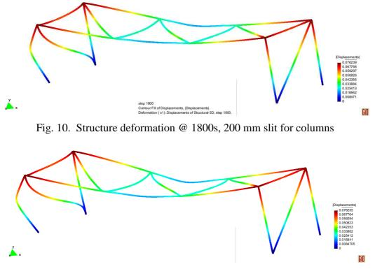
Fig. 11. Structure deformation @ 1800s, 20 mm slit for columns
