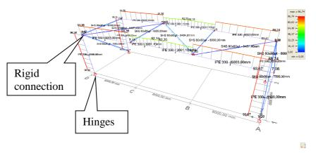
Fig. 2. Reference case, unity check at ambient temperature
