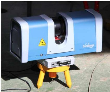
Fig. 6 Laser scanner
