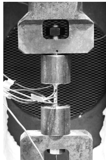
Fig. 2 Test setup for turned-down bolt specimen.
