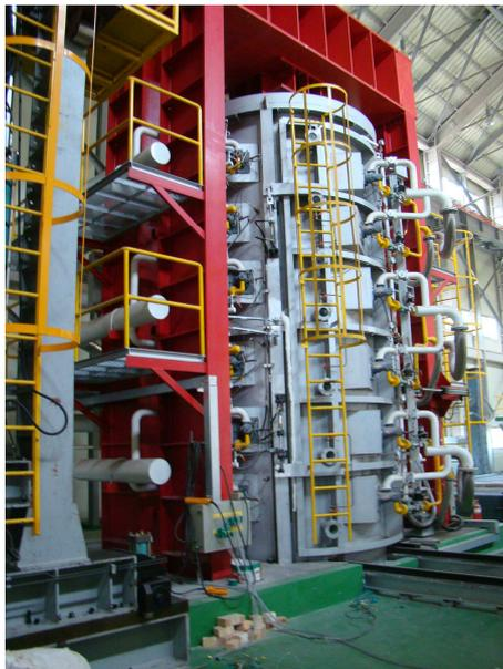
(a) 10,000 kN heating furnace
