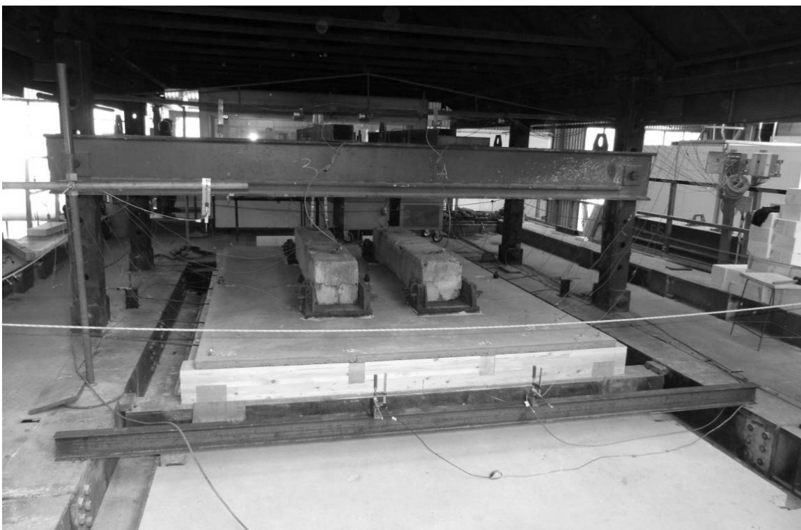
Fig. 1 Fire test set-up
