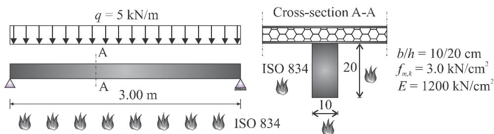
Fig. 5 Data for simply-supported timber beam
