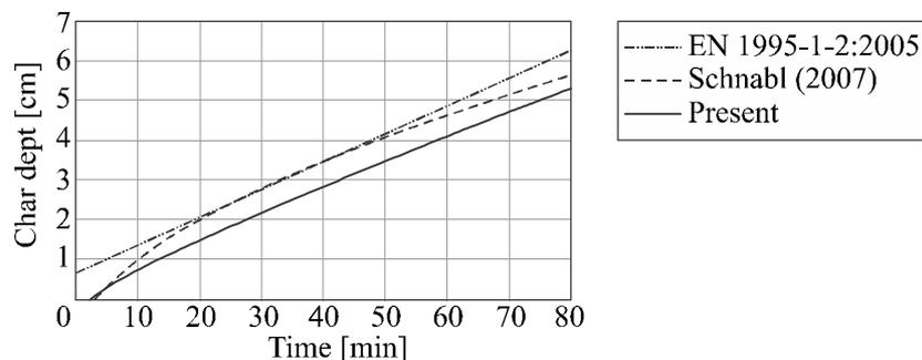
Fig. 4 Comparison of different one-dimensional charring models
