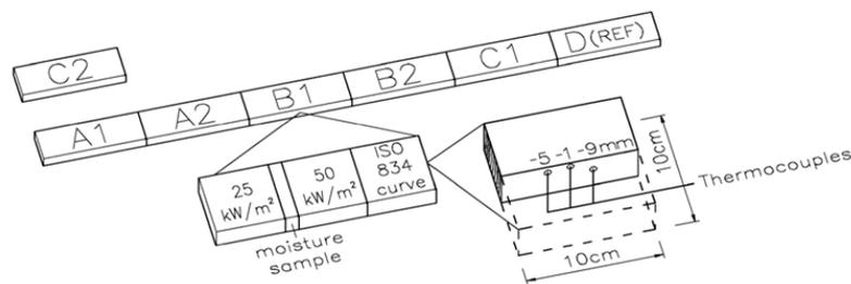
Fig. 1 Schematic representation of the sample preparation procedure
