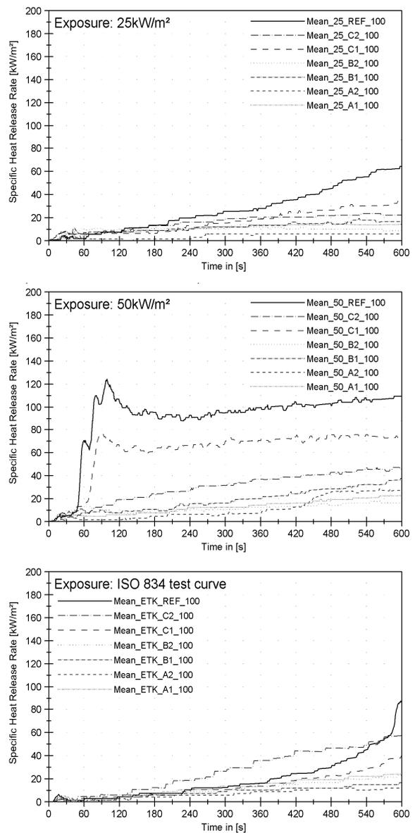
Fig. 4 Rate of heat release curves (mean value of 3 replications) during the cone test with the irradiance of  $25 \text{ kW/m}^2$ ,  $50 \text{ kW/m}^2$  and the standard ISO curve for the test duration of 600 s for the different fire retardant products and the untreated reference series
