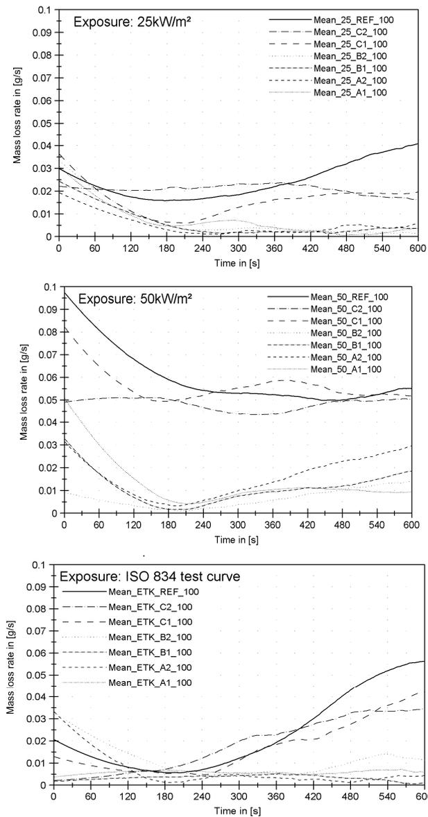
Fig. 3 Mass loss rate curves (mean value of 3 replications) during the cone test with the irradiance of  $25 \text{ kW/m}^2$ ,  $50 \text{ kW/m}^2$  and the standard ISO 834 curve for the test duration of 600 s for the different fire retardant products and the untreated reference series
