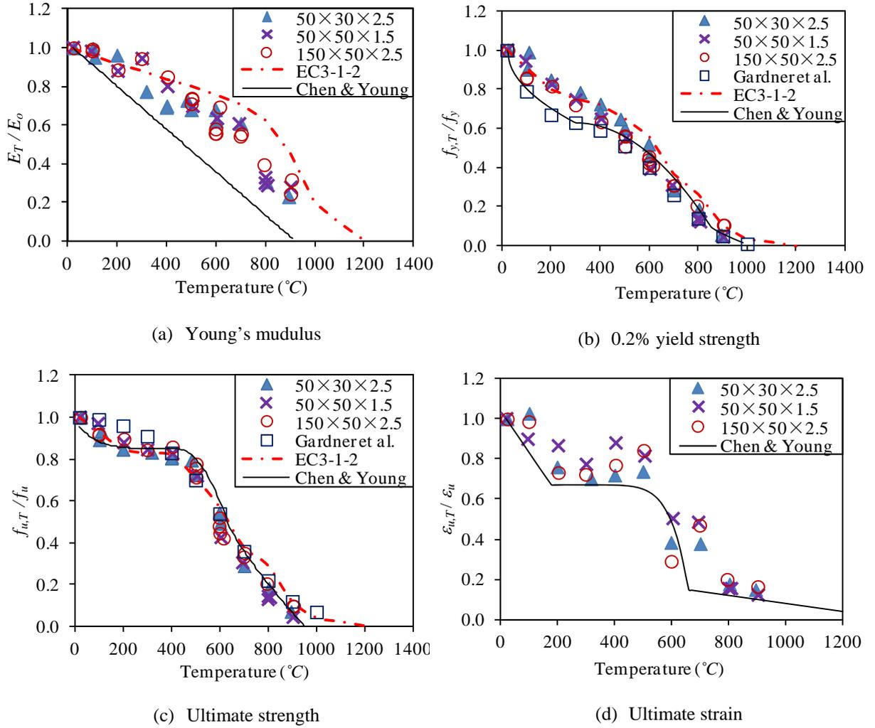
Fig. 3: Comparison of material properties obtained from design rules and test results
