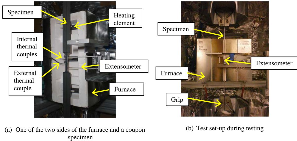
Fig. 2: Typical test set-up of a coupon specimen
