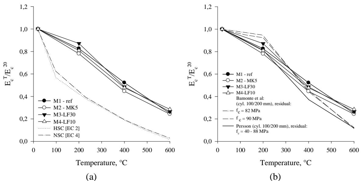
Fig. 2 Plot of the relative secant modulus of elasticity vs. temperature: a) this study and models in EC2 and EC 4 and b) this study and results in Persson, 2004 and Bamonte 2012
