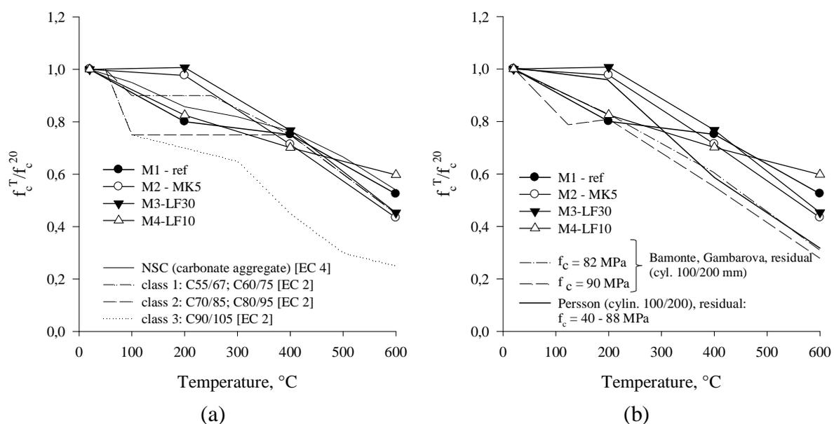
Fig. 1 Plots of the residual compressive strength vs. temperature: a) this study and models in EC2 and EC4 and b) this study and results in Persson, 2004 and Bamonte 2012
