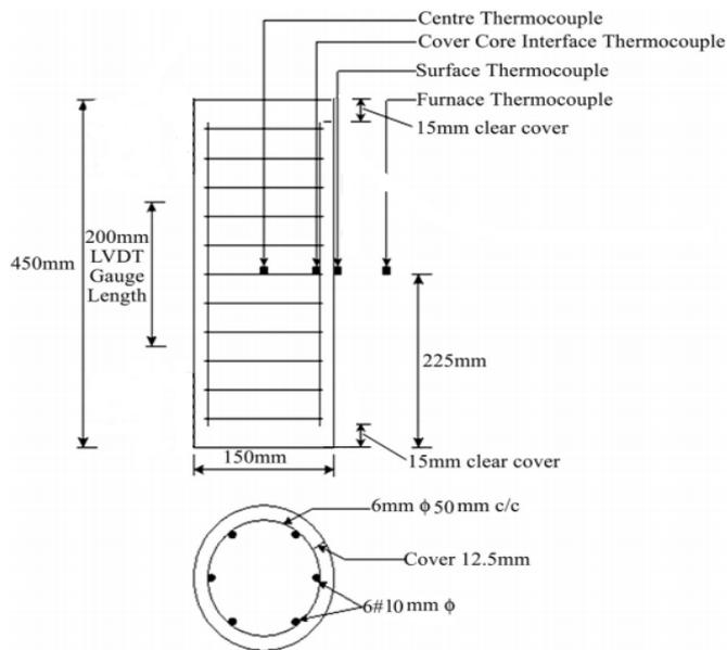
Fig. 1 Reinforcement details and position of thermocouple
