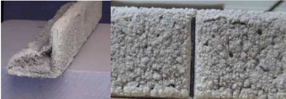
Fig. 4. L-section after firth test
