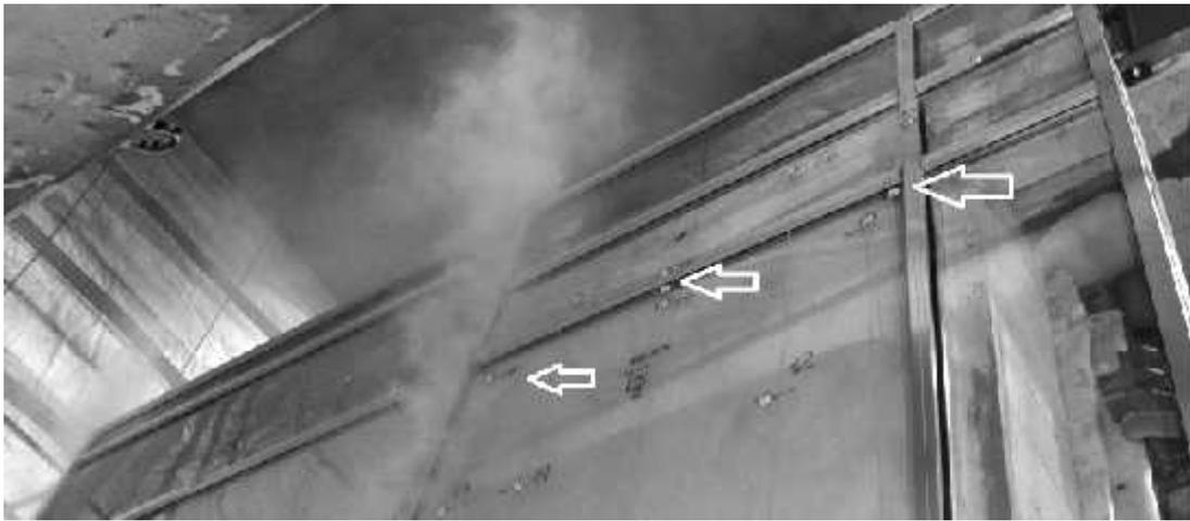
Fig. 4 Additional thermocouples placement in fire resistance test of curtain wall, test 2
