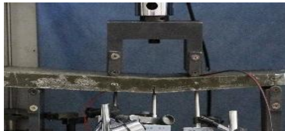
Fig. 1 - Four-point bending test
