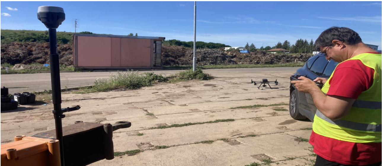
Fig.2 - Preparation by DJI M300, Emlid RS3 base station and 3gon Positioning worker, photo by O.Váňa
