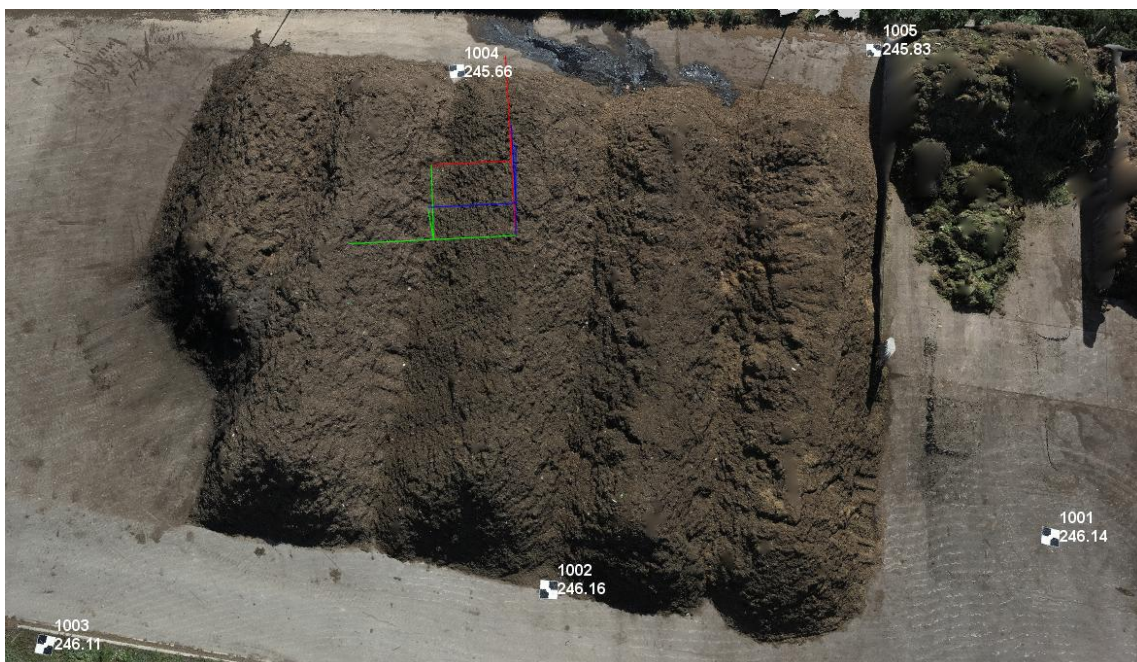
Fig.9 - Placement of Ground Control Points, by O. Váňa
