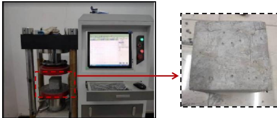
Fig. 2 – ECC compression test device
