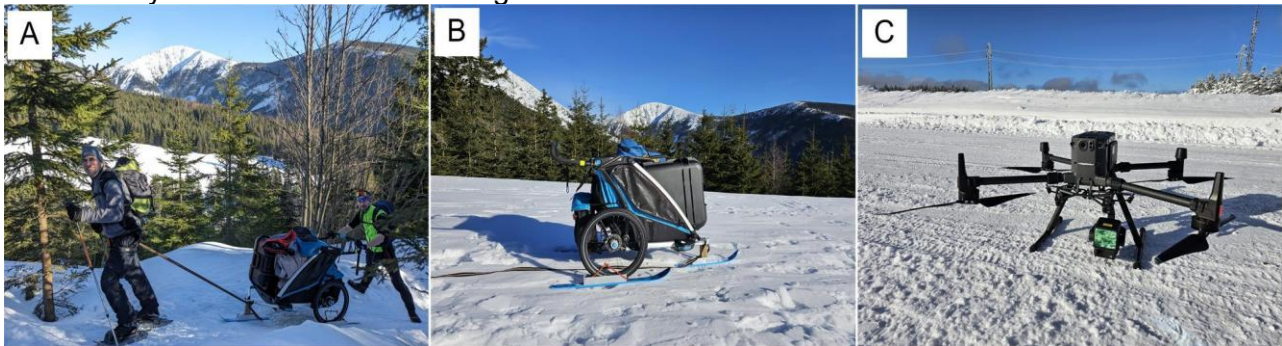
Fig. 2 A and B - drone transportation in the mountainous area; C - DJI Matrice 300 RTK equipped with Zenmuse L2 LiDAR scanner
