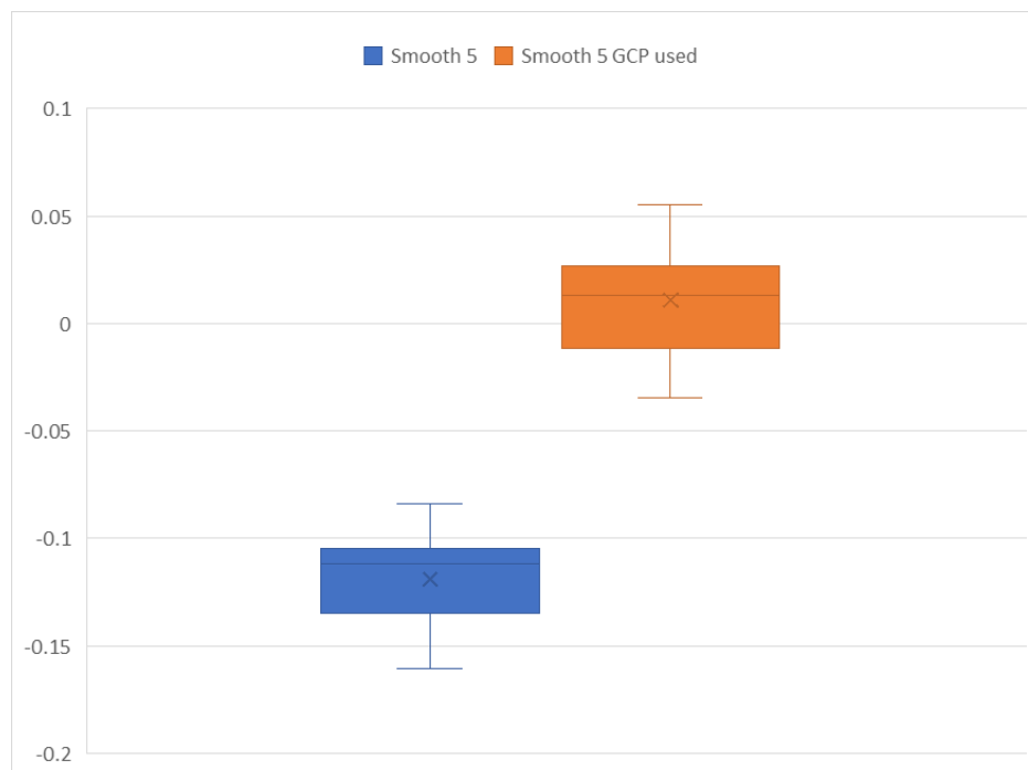
Fig. 6 Box plot of errors in Z coordinate on point cloud without Ground Control Point co-registration (blue) and with Ground Control Point co-registration (right).
