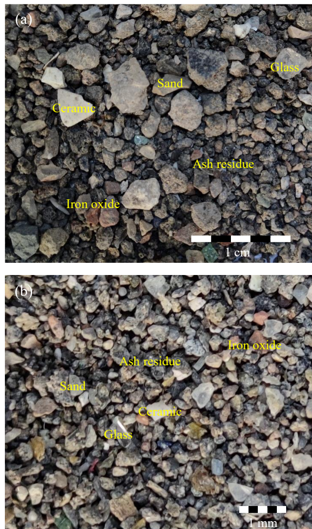
Fig. 2 - Particles of MSWI bottom ash. (a) \geq 2.36 mm; (b) 0.6–1.18 mm
