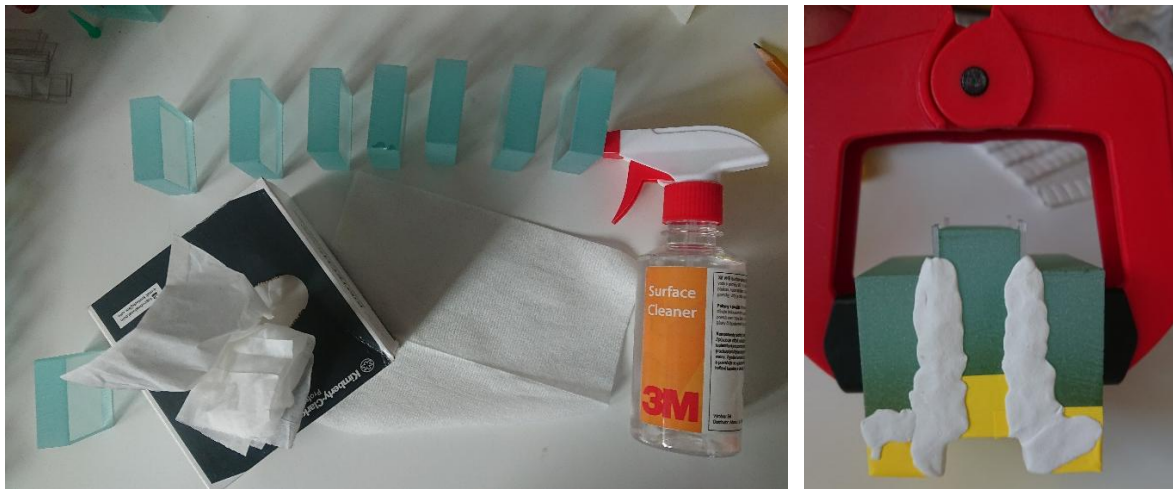
Fig. 3 - Cleaning of the glass panes (left), specimen prepared for bonding (right)
