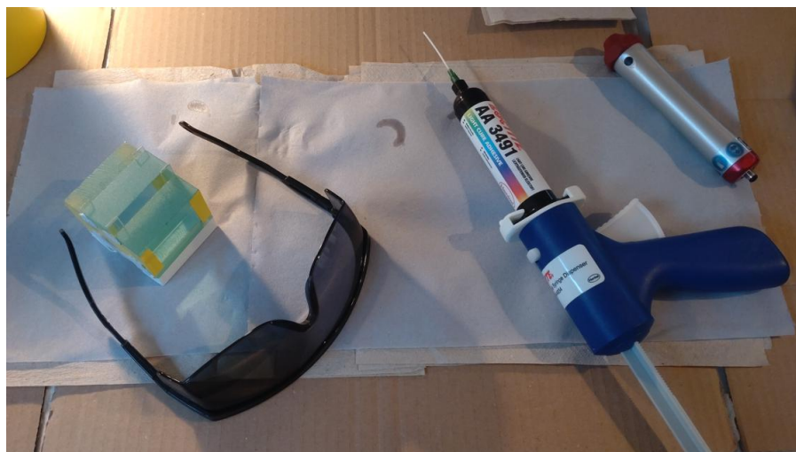
Fig. 4 - Set-up for bonding specimen with UV adhesive - from left: specimen secured by tape, UV protecting glasses, UV adhesive with dispenser gun and application needle, LED spot
