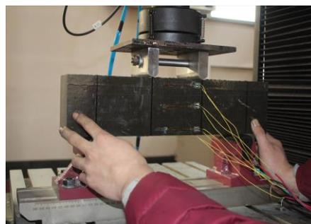
Fig. 3 - Bending test for PUC material
