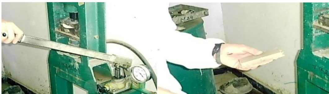
Fig. 6 – Manufacture of pressed bricks
