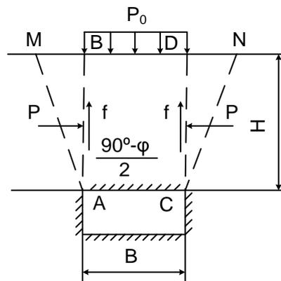
Fig.3- Schematic diagram for roof stability of Goaf
