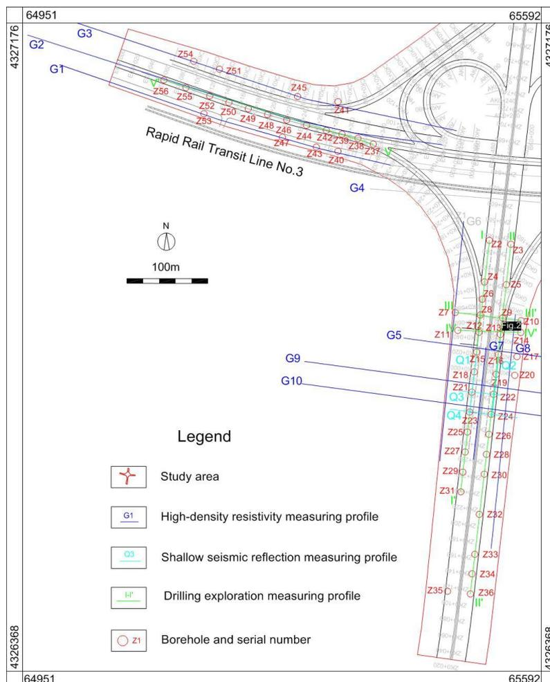
Fig.5 - Map of an engineering geological exploration
