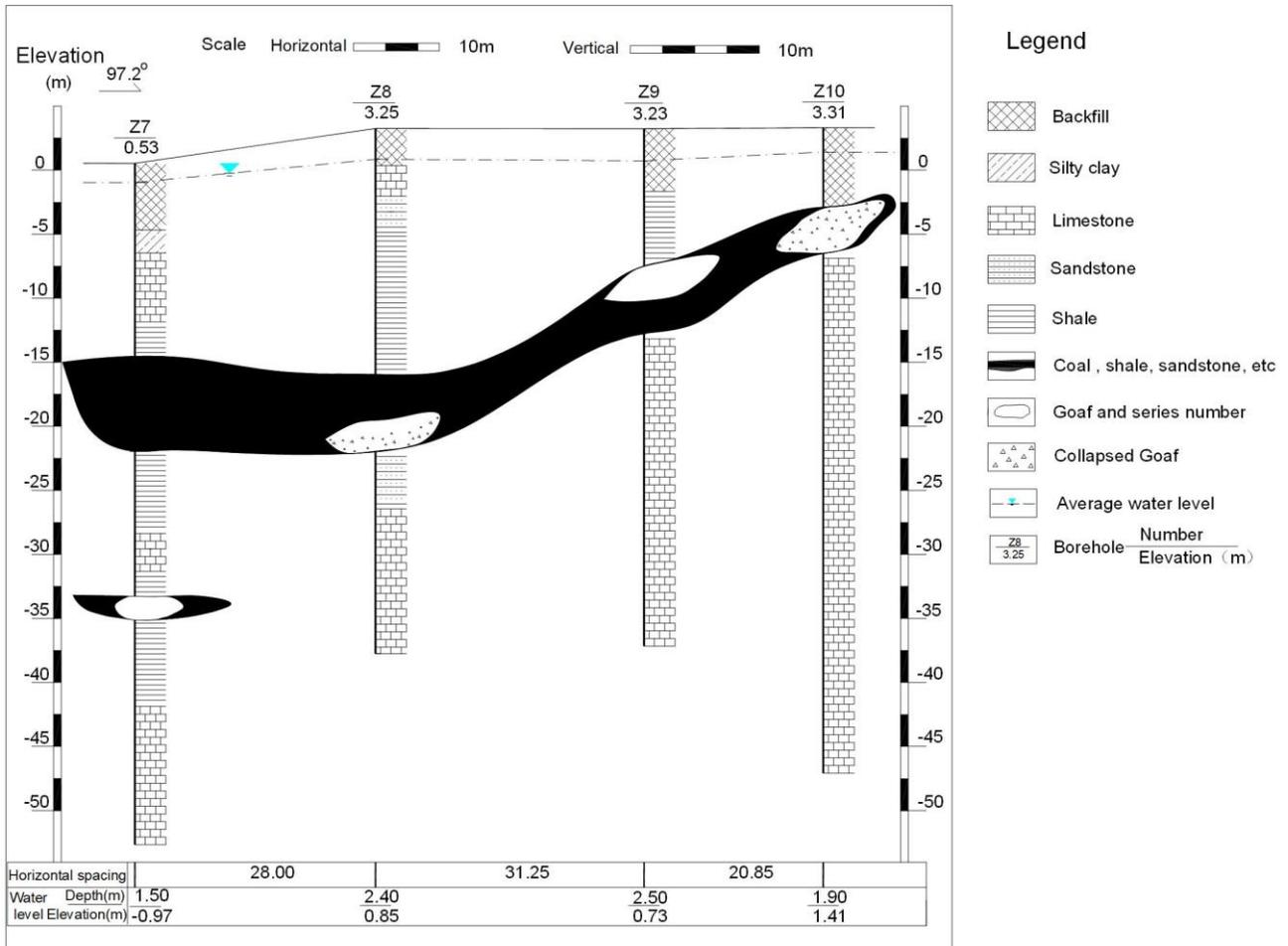
Fig.8- III-III' engineering geological profile
