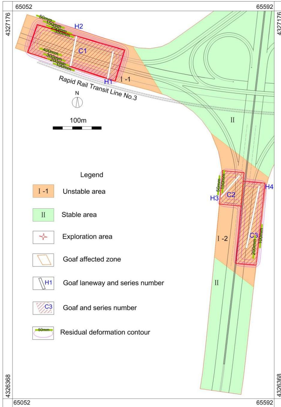
Fig.10- Distribution of Goafs for the No.9 Line Overpass across Rapid Rail Transit Line No.3 and zoning of surface stability
