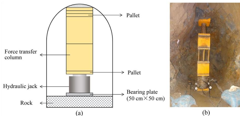
*Fig. 4 - The load test, (a) Test schematic diagram, (b) Test photos*
