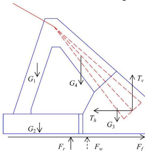
Fig. 9 - Force diagram of the gravity anchorage
