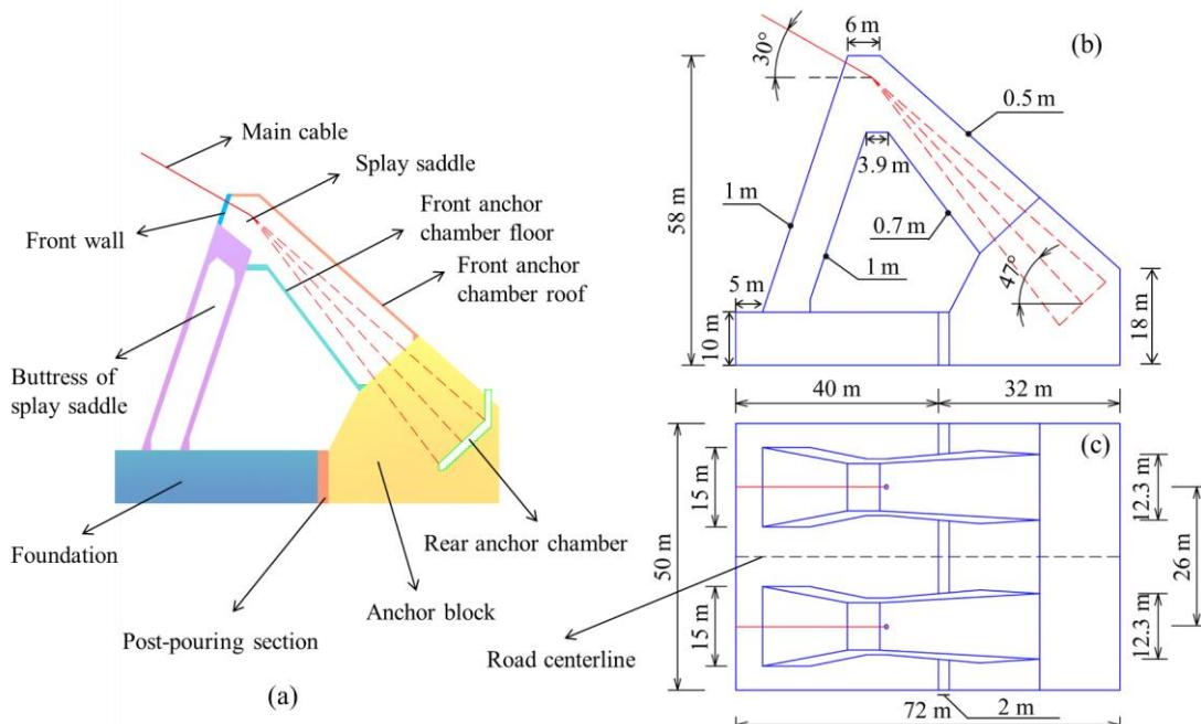
Fig. 2 - Composition and size of the gravity anchorage, (a) The main structure of the gravity anchorage, (b) Elevation of the gravity anchorage, (c) Top view of the gravity anchorage
