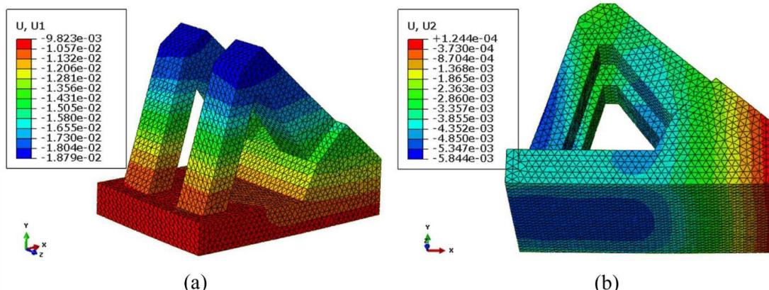
Fig. 11 - The horizontal and vertical displacements of the gravity anchorage (unit: m), (a) Horizontal displacement of the gravity anchorage, (b) Vertical displacement of the gravity anchorage
