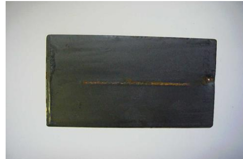
(d) Coal tar epoxy coating with 1 wt.% anion exchange cellulose in NO_3^- form
