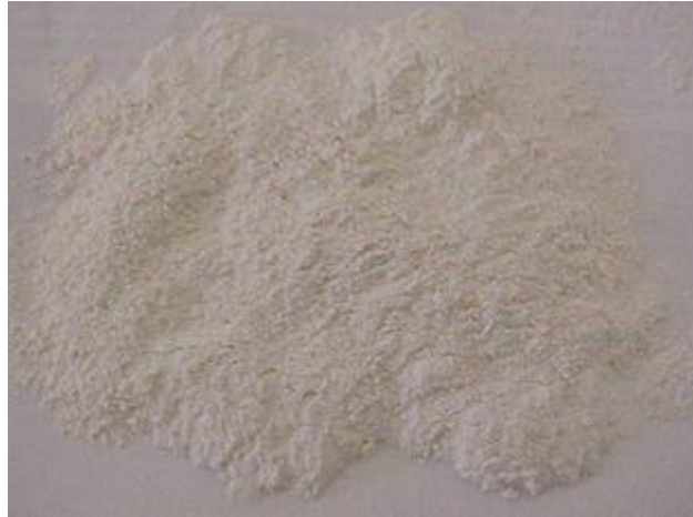
Fig. 2 - An example biobased ion exchanger (anion-exchange cellulose in \text{SO}_3^- form) after ball milling.
