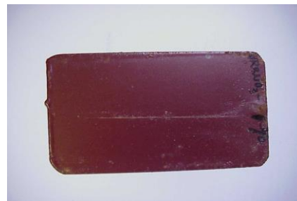
(b) Vinyl coating with 1 wt.% anion exchange cellulose in \text{NO}_3^- form
