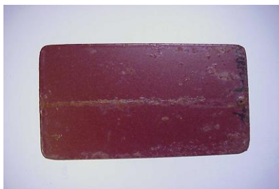
(a) Vinyl coating with 1 wt.% anion exchange cellulose in \text{PO}_4^- form
