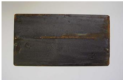
(c) Coal tar epoxy coating with 1 wt.% anion exchange cellulose in SO_4^- form
