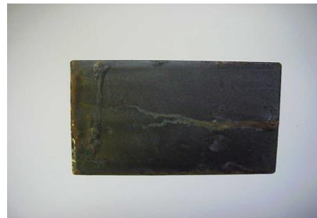
(d) Coal tar epoxy coating with anion exchange cellulose in NO_3^- form
