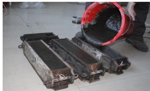
*Fig. 2- Pouring drawing of PUC*
