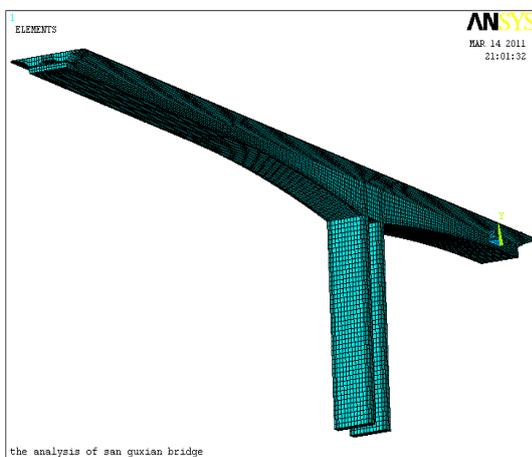
Fig. 3 – Finite element model of bridge
