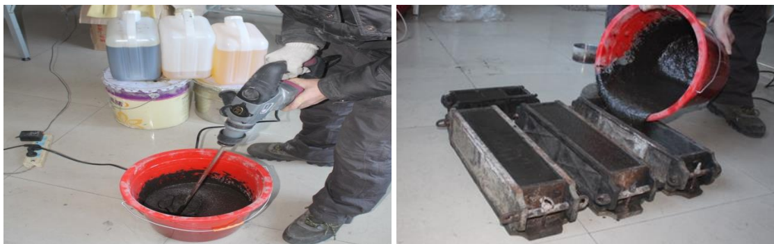
Fig. 1 - PUC material mixing diagram
