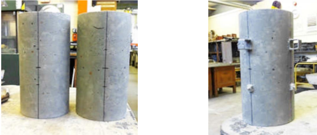
Fig. 9 – Samples for testing elasticity modulus
