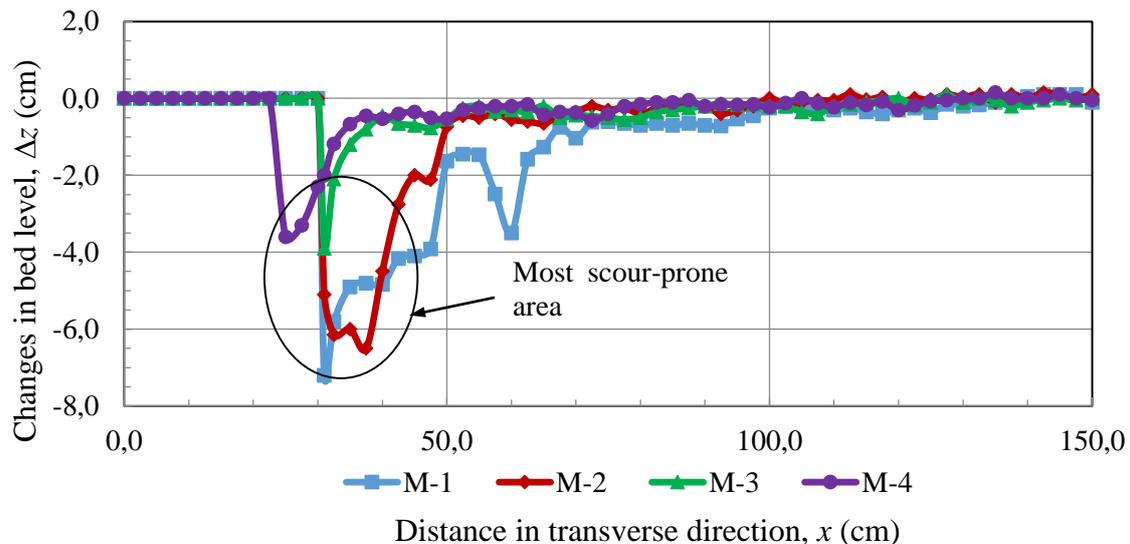
Fig. 8 – Bed level changes along the cross-section at the first groin
