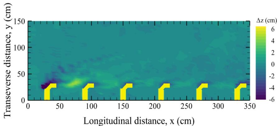
Fig. 6 – Model M-3 induced bed topography
