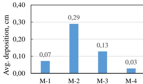
Fig. 10 – Average deposition in the groin field due to various groins
