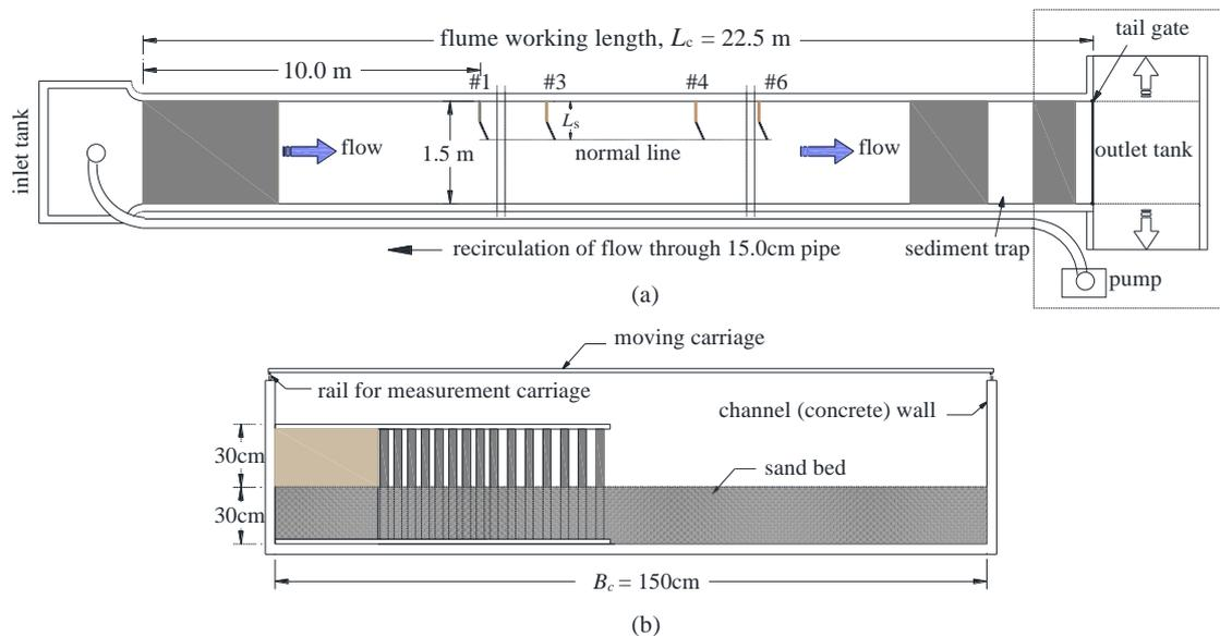
Fig. 1 – Laboratory channel: (a) Plan view; (b) Cross-section
