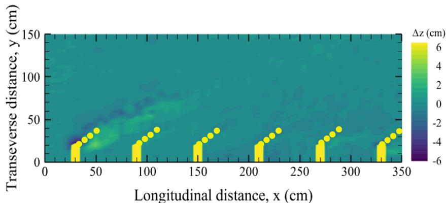
Fig. 7 – Model M-4 induced bed topography
