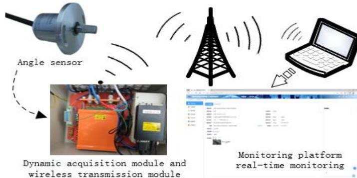
Fig.7 - Angular velocity acquisition process
